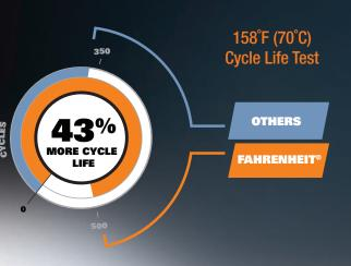
J2185 Test at 158°F with charging at 14.2 volts. Others based on 2 part number 2 sample average. Fahrenheit on 2 sample average
